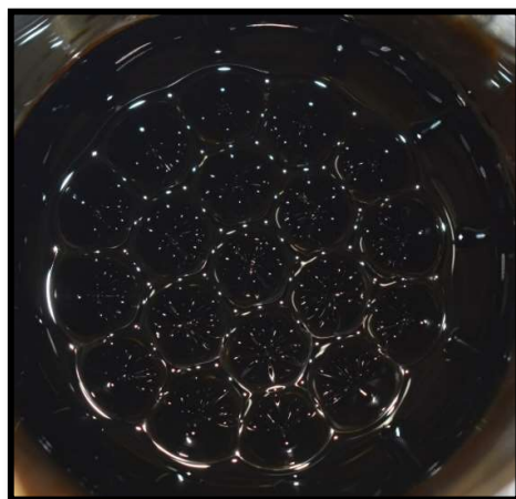
Figure 3.1 Rosensweig instability possessed by a hydrocarbon based ferrofluid in the presence of a uniform magnetic field
