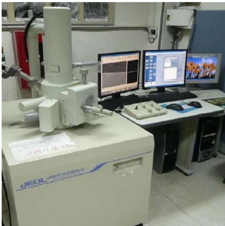
Fig 2.5 SEM machine used for the measurement( Jeol 6390LA/ OXFORD XMx N)
