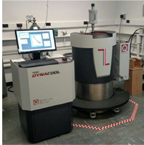
Fig 2.7. Illustration of Vibrating Sample Magnetometer and Quantum Design Physical Property Measurement System (PPMS)
