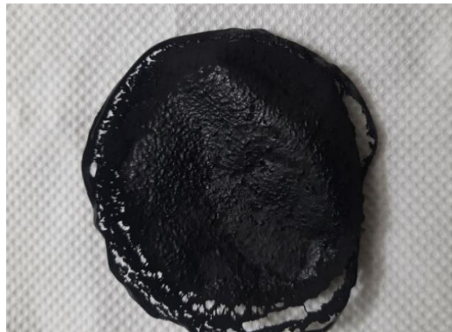
Figure 3.11 Photograph depicting the PVA-CB metacomposite film (PC7) fabricated with 3 wt% CB. As observed the film is non-uniform owing to the aggregation of CB on the surface
