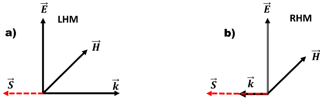
Figure 1.3 (a) Double negative materials (DNG), (b) Double positive materials (DPS)
