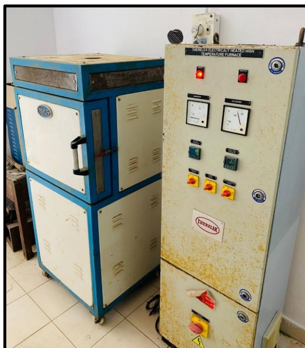
Figure 2- 2 High temperature furnace ( T_{\max}=1700\text{ }^{\circ}\text{C} ) with PID programmable controller and molybdenum disilicide ( \text{MoSi}_2 ) heating elements.
