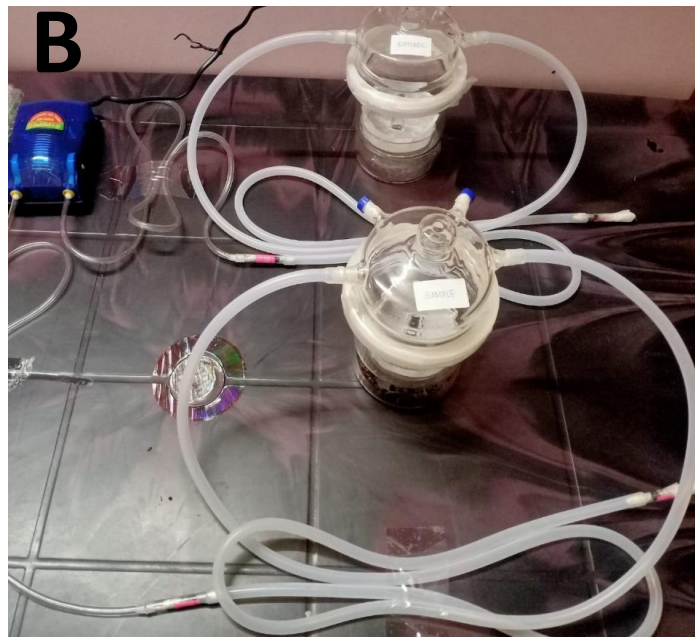
Figure 3.4. A- The picture depicts an economically feasible glass chamber designed to conduct the whole body volatilome of insects. This chamber has 2 inlets and 2 outlets to facilitate the movement of volatile compounds along with air pushed through the system. The separation disc prevents the unnecessary movements of the beetle through the chamber. B- Figure represents the experimental setup. Air was pumped after filtering through activated charcoal to the inlet, which collects the air containing volatiles from beetles and pushes them to the activated charcoal adsorbent attached to the outlet.
