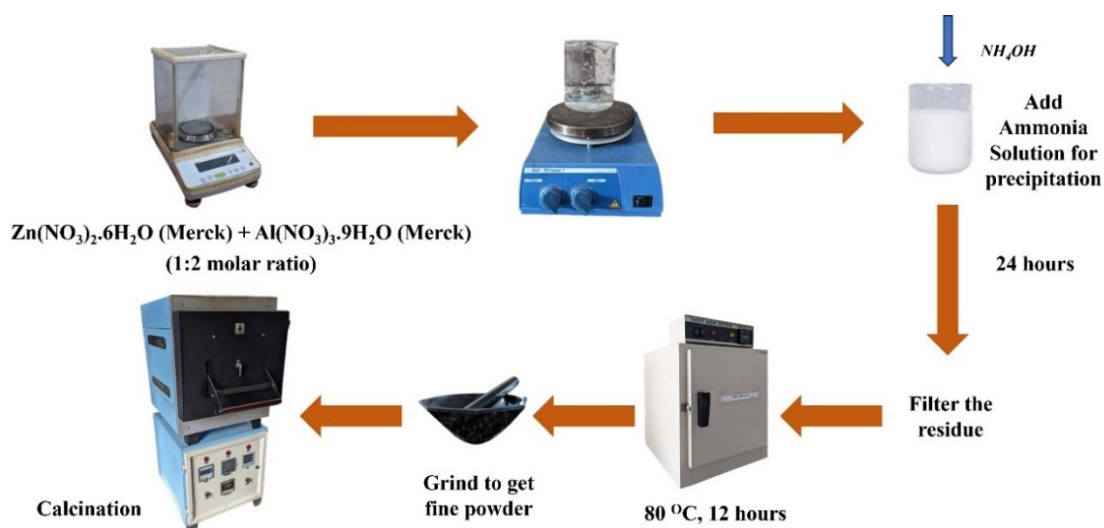
Fig 2.2 Flow chart of co-precipitation method
