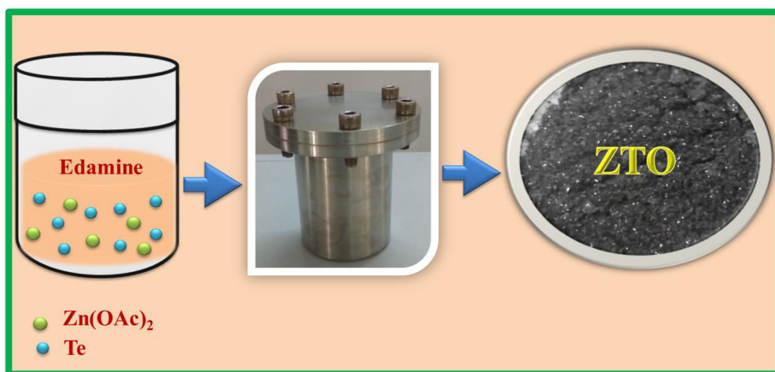
Figure 6.1 Flow chart of the synthesis of ZTO
