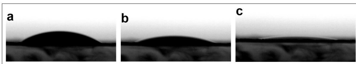
Fig 6.17 Contact angle of ZTO (a) initial (b) within hundred seconds (c) after 2 minutes
