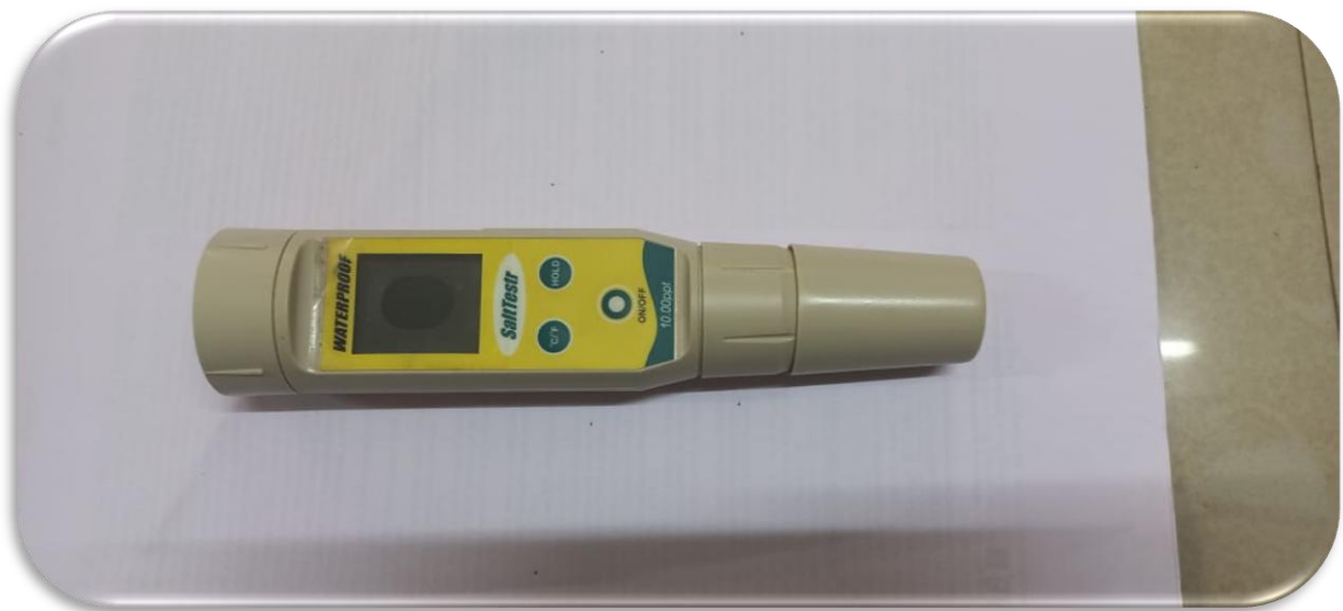
Fig.10 salinometer used to determine the salinity of the sample
