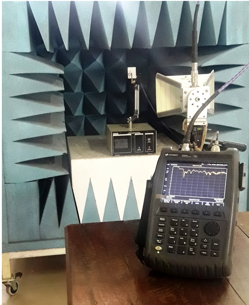
Figure 5.9: Photograph of the experimental set up for the radiation pattern measurement of monopole antenna.
