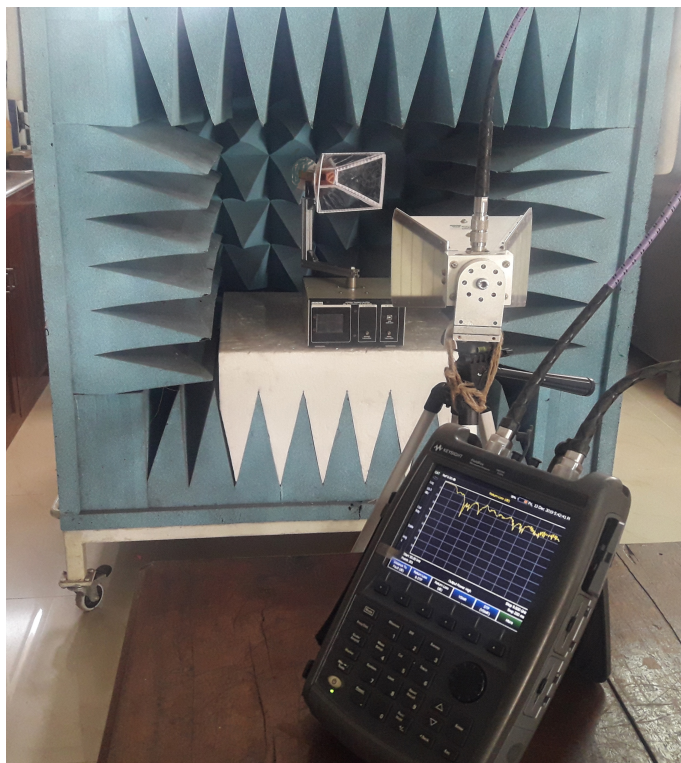
Figure 4.7: Experimental setup showing the radiation pattern measurement of AUT placed in a anechoic test box using VNA and wide band dual ridge horn as transmitter.
