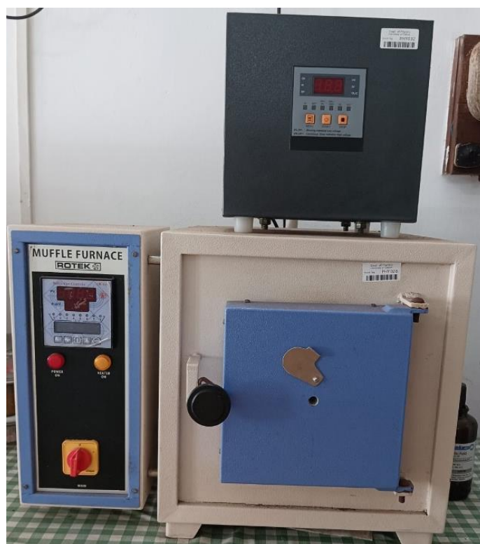
Fig. 2.1 Image of the muffle furnace used in the study (located at the Laboratory for Mesoscopic Sciences and Devices, Department of Physics, University of Calicut).
