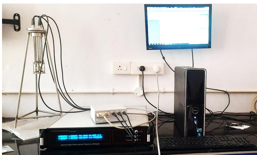
Fig. 2.5 (a) Schematic diagram of the BDS Analyzer [11] (b) Image of Model Novocontrol BDS Analyser- Department of Physics, University of Calicut (used for analysis in the thesis).
