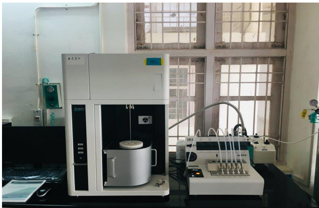
Fig. 2.4 (a) Schematic diagram of the BET surface area analyser [6], (b) Image of Model BELCAT-M– CSIF University of Calicut (used for analysis in the thesis) [3].
