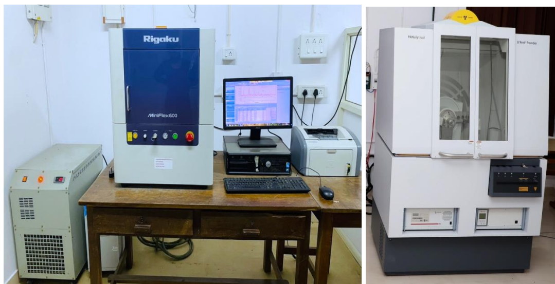
Fig.2.2 (a) Schematic diagram of XRD (image adapted from [2]). (b) Image of Rigaku Miniflex 600 X-ray Diffractometer-Department of Physics, University of Calicut. (c) X'pert 3 Powder X-RAY Diffractometer-CSIF University of Calicut [3] (used for analysis in the thesis).
