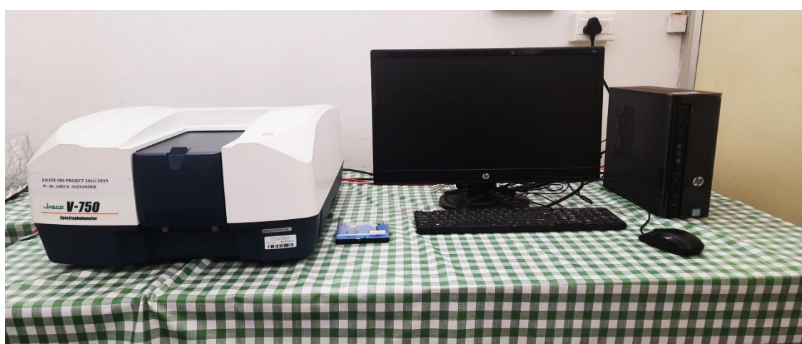
Fig. 2.7 (a) Schematic diagram of the UV-Visible Spectrometer set-up [18], (b) UV-Visible Jasco V-750 spectrophotometer Department of Physics, University of Calicut (used in this study).
