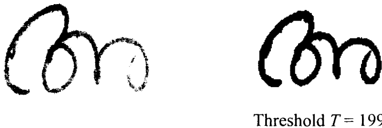
Figure 4.4 Input gray-scale image and its binary output obtained using Otsu's technique
