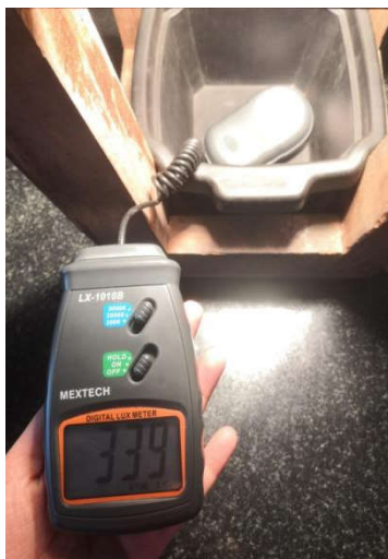
Figure 5.12 Light intensity measuring using Digital lux lumen meter
