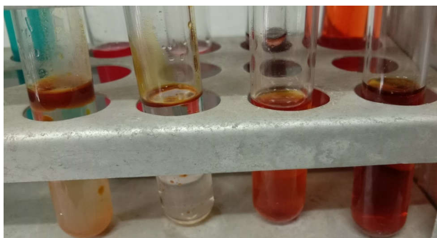
Figure 5.6. Extraction of congo red dye with hydrophobic ILs (1) [P_{14,6,6,6}][Cl] IL, (2) [P_{14,6,6,6}][N(CN)_2] IL, (3) [P_{14,6,6,6}][NTf_2] IL & (4) without treating IL
