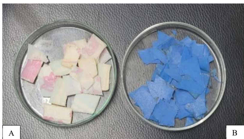
Fig. 7.3 Degradation image of A) Sanitary napkin and B) Polycoated paper carry bag after week 4.
