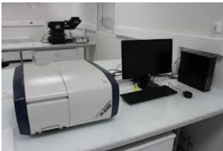
Figure 2.14: FP-8300 JASCO spectrofluorometer with an excitation wavelength of 330 nm used for PL measurements.
