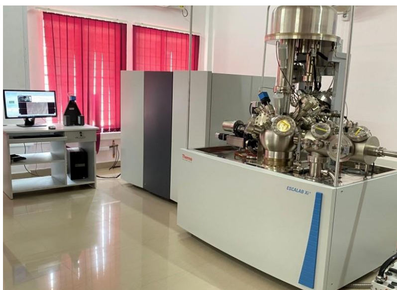
Figure 2.7. Thermo Scientific ESCALAB equipment equipped with Al K \alpha monochromator
