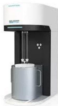
Figure 2.17: BET surface area, pore volume, pore diameter analyzer: BELSORP-MAX instrument.
