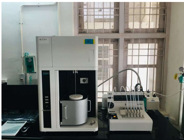
Figure 2.11 Image of BET instrument at CSIF, University of Calicut.
