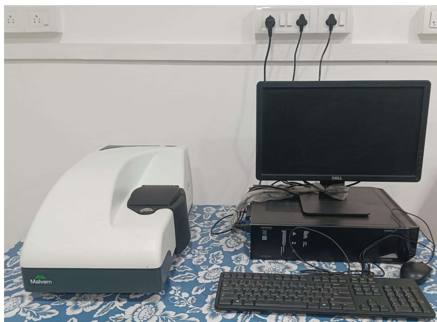
Figure 2.15 Image of DLS instrument at Department of Nanoscience and nanotechnology, University of Calicut
