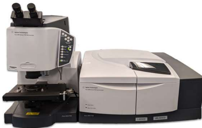
Figure 2.16 FTIR Spectrometer. Image adapted from [110]
