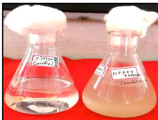
Fig.5.1 The enrichment of formulated bacterial consortium in a mineral salt medium for four months by adding bacterial cultures to a conical flask and comparing results with its control conical flask without bacterial inoculation.
