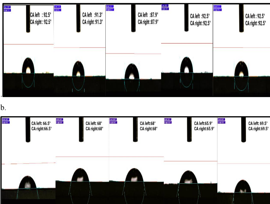
Fig.4.6(a) WCA measurements of Bacillus cereus NJD1. a. Video captured images (five in number) of LDPE films without bacterial addition, inoculated in the synthetic, carbon-free medium for 120 days. b. WCA images of Bacillus strains inoculated on LDPE films.
