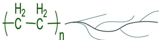
Fig 2.4 Chemical structure and branching nature of LDPE (C_2H_4)_n
