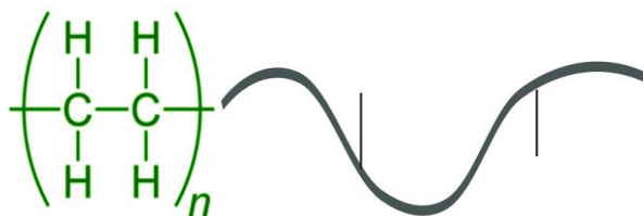
Fig. 2.2 Chemical structure and branching nature of HDPE with empirical formula (C_2H_4)_n
