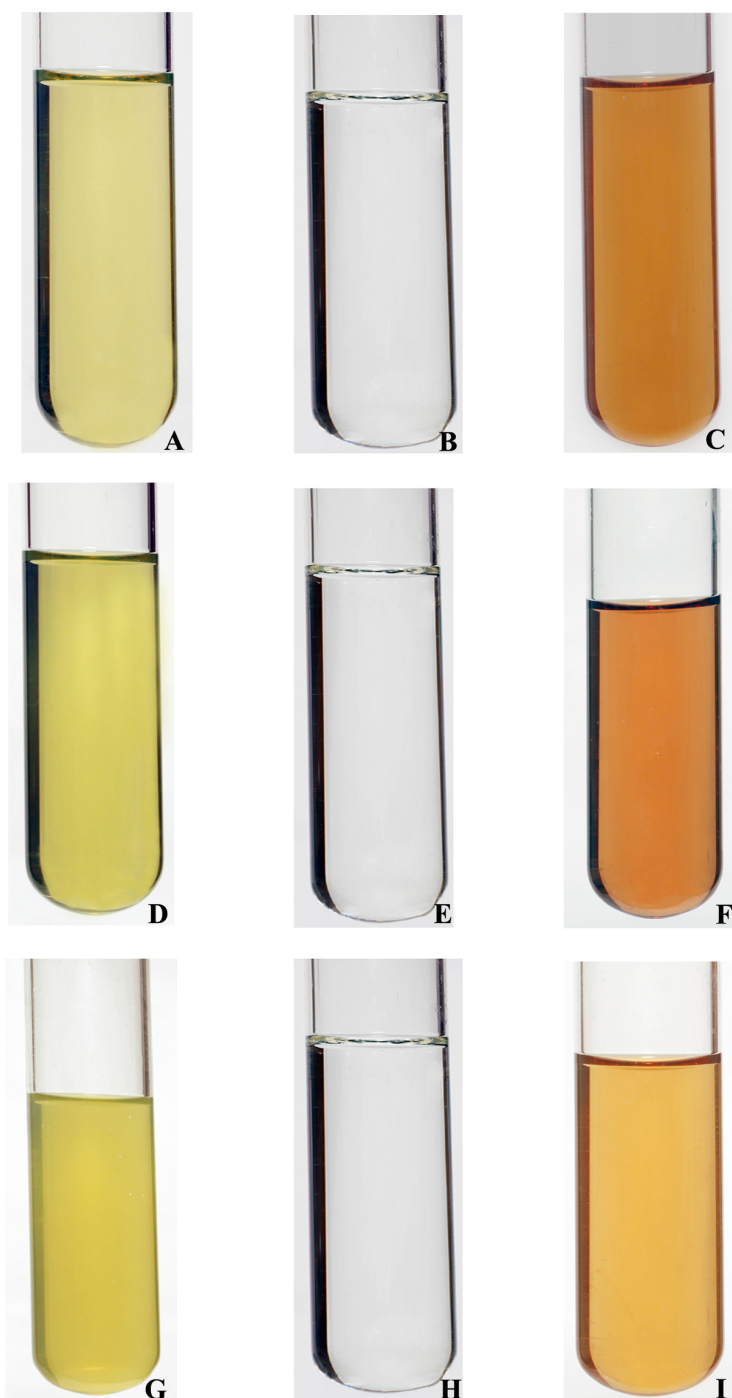
Green synthesis of silver nanoparticles. A, D, G: GHH, GHR and GE solutions before the synthesis of silver nanoparticles B, E, H: 2 mM silver nitrate solution C, F, I: GHH, GHR and GE solutions after the synthesis of silver nanoparticles. GHH - G. heyneanum var. heyneanum ; GHR - G. heyneanum var. rottleri ; GE - G. eriocarpum
