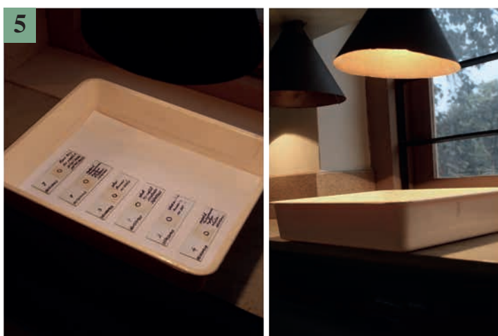
5. Drying of microscopic slides under incandescent bulb.
