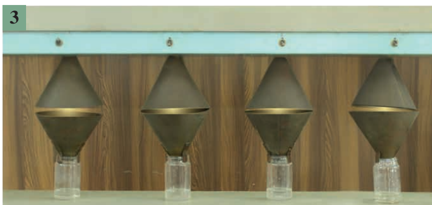
3. Mite extraction using Berlese-Tullgren funnel apparatus.
