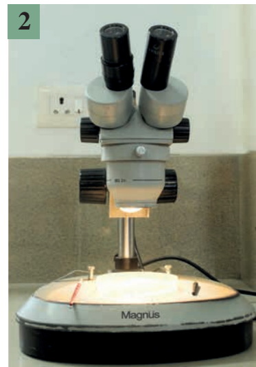
2. Direct mite extraction under stereozoom microscope.
