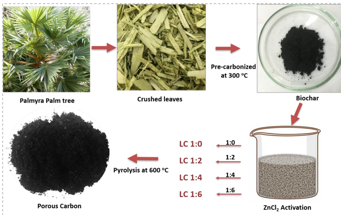
Figure 6.20. Schematic illustration of ZnCl 2 activated highly porous carbon formation from palm leaf by pyrolysis at 600 °C
