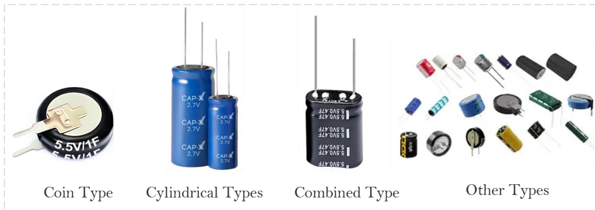
Figure 1.3 Supercapacitor arranged in different types based on their application and usage*
