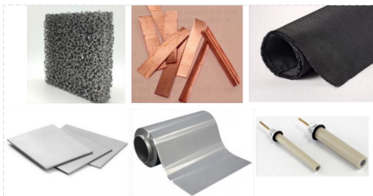
Figure 1.10 Images of various commercially available current collectors for supercapacitor fabrication like nickel foam, copper sheet, carbon cloth, graphitic plate, stainless steel and glassy carbon electrode*
