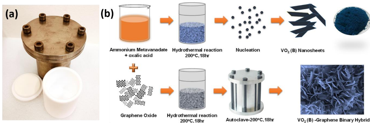
Figure 2.2 (a) A photograph of stainless-steel autoclave with teflon liner used for the hydro/solvothermal process and (b) representation of metal oxide synthesis using hydrothermal method
