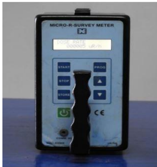
Figure 3.1: Micro-R survey metre.
