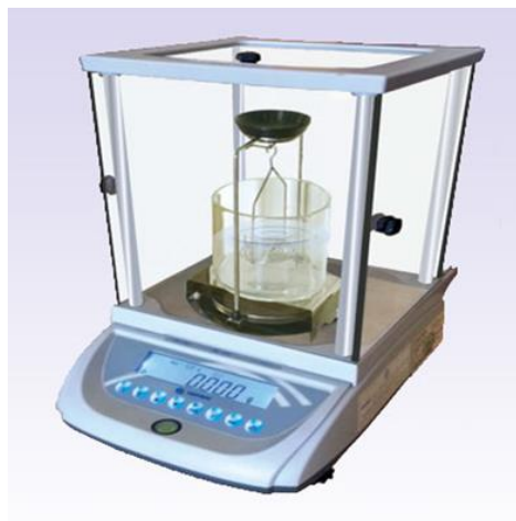
Figure 7.4: Density kit with balance
