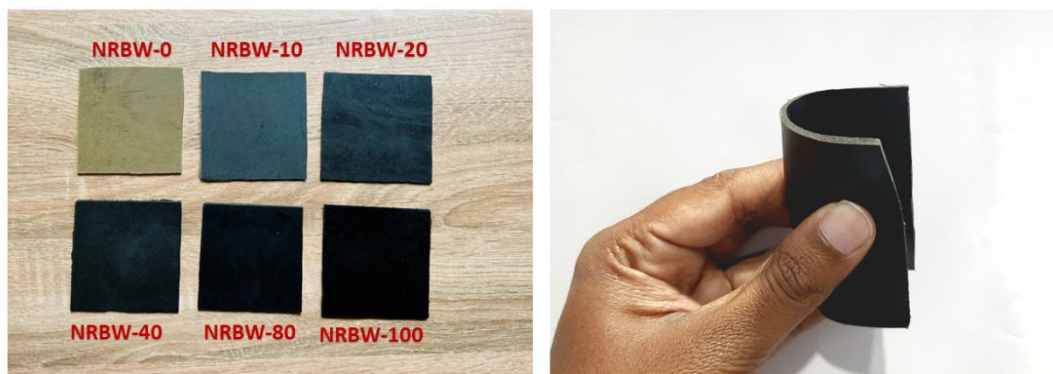
Figure 7.6: The fabricated flexible NR composites with NRBW nanoparticles.
