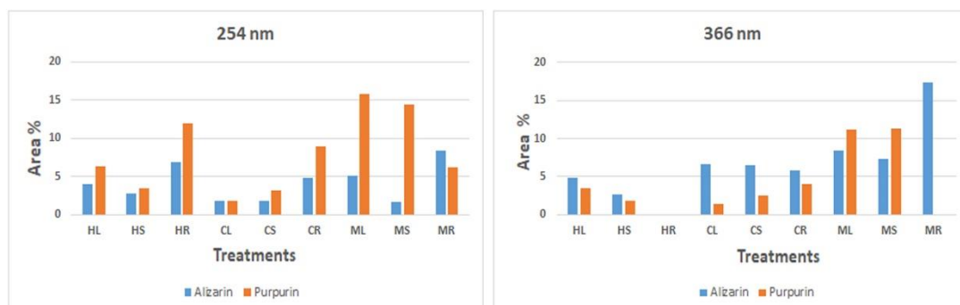
Figure 4: The HPTLC analysis of R. cordifolia grown in vitro , extracted using different solvents; HL-Hexane leaf, HS-Hexane stem, HR-Hexane root, CL-Chloroform leaf, CS-Chloroform stem, CR-Chloroform root, ML-Methanol leaf, MS-Methanol stem, MR-Methanol root
