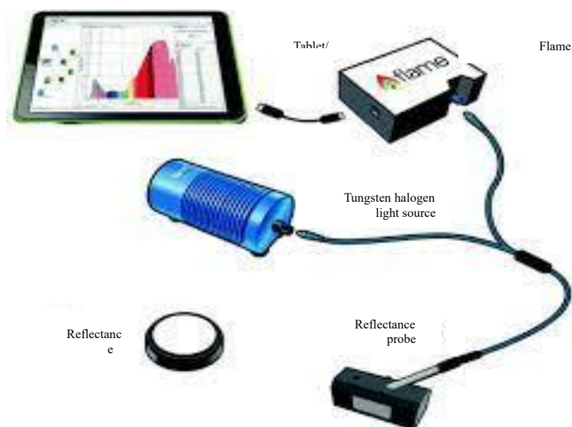
Fig 2.14 The experimental setup used for the reflectance measurement [55]
