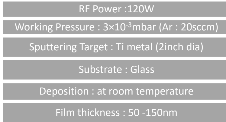
Fig. 4.2 Deposition conditions of titanium metal films
