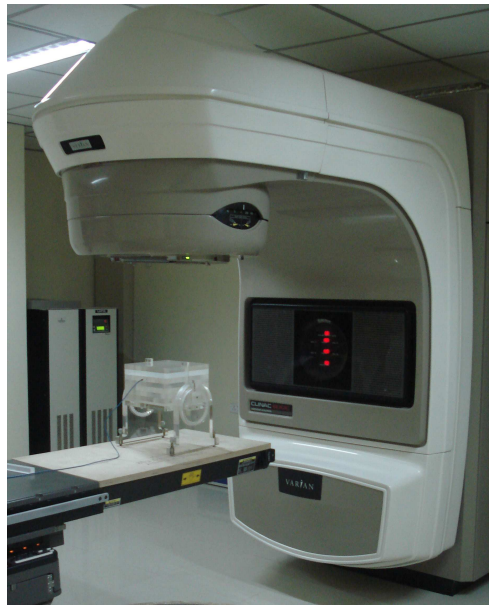
Figure 5.15. Experimental setup of PMMA phantom in linear accelerator
