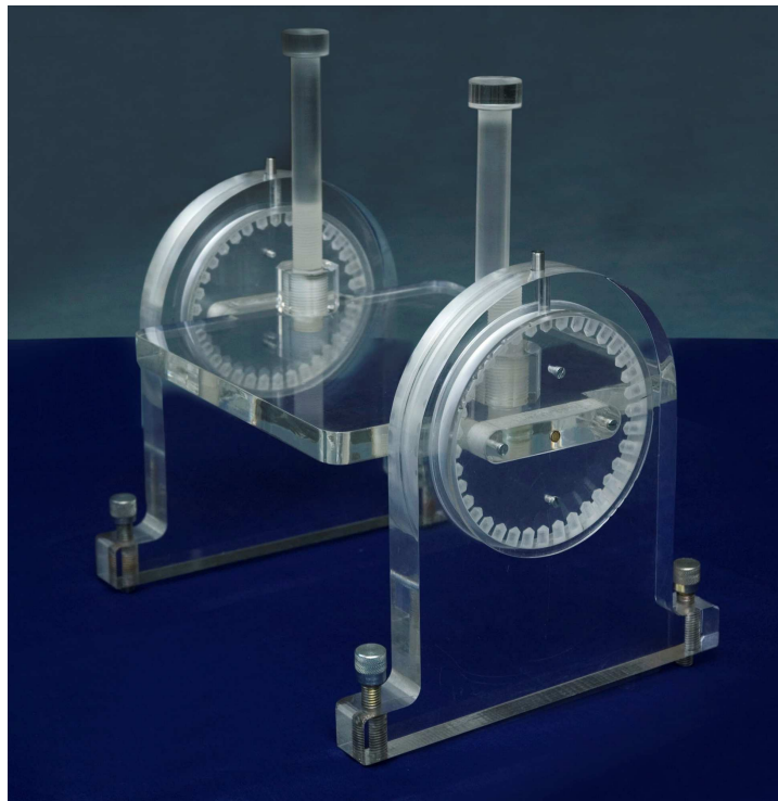
Figure 4.5 Stacking frame assembled from fabricated parts
