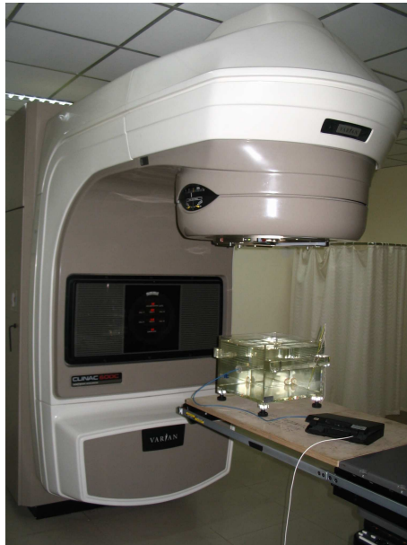
Figure 5.16. Experimental setup of water phantom in linear accelerator
