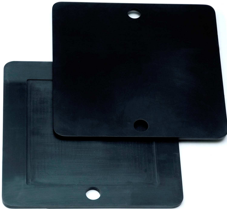
Figure 4.6 Fabricated Film holder with black PMMA
