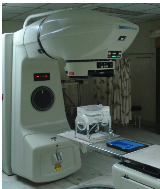
Figure 5.14. Calibration setup in Cobolt-60 teletherapy machine
