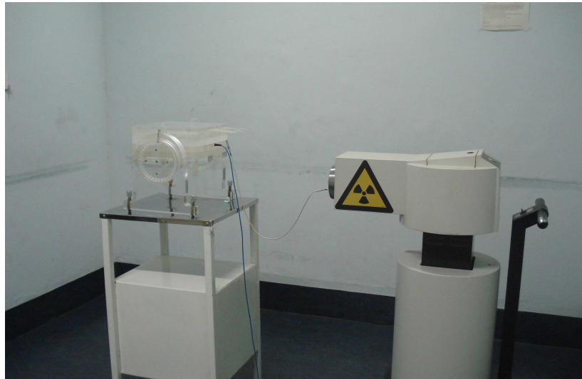
Figure 5.9. Experimental setup of phantom with HDR plate and cylindrical ionization chamber in HDR machine
