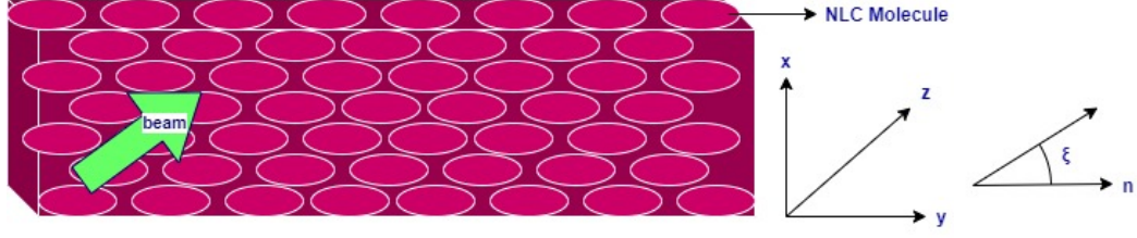
Figure 3.1: The interaction geometry. A nematic liquid crystal with ellipses which have long axes parallel to y is used to represent the elongated NLC. The input light beam is shown with a green arrow impinging normally to the molecular director on the sample. The angle \xi describes the reorientation of the optic axis, n in the (x, y) plane.
