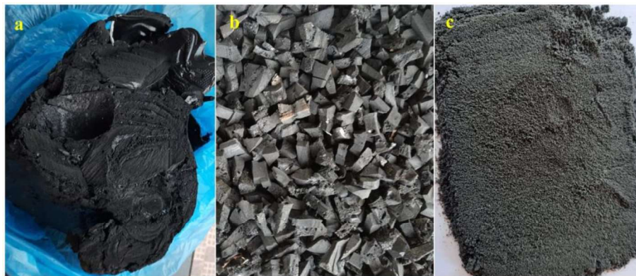
Figure 2.2. Digital images of (a) PUW, (b) cut pieces of PUW and (c) powdered PUW
