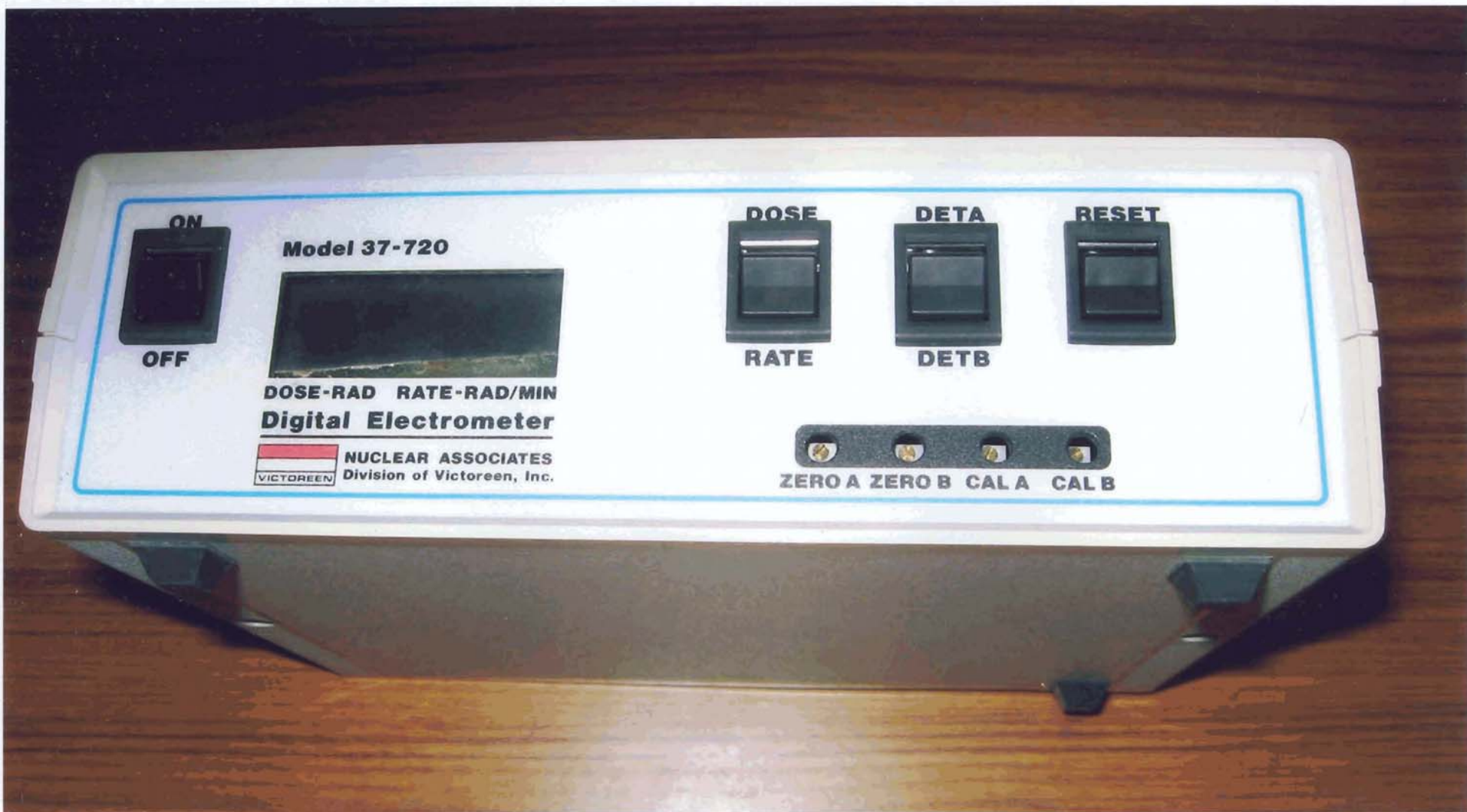
Figure 13 - Digital electrometer to read the dose absorbed by the dosimeters in cGy.
