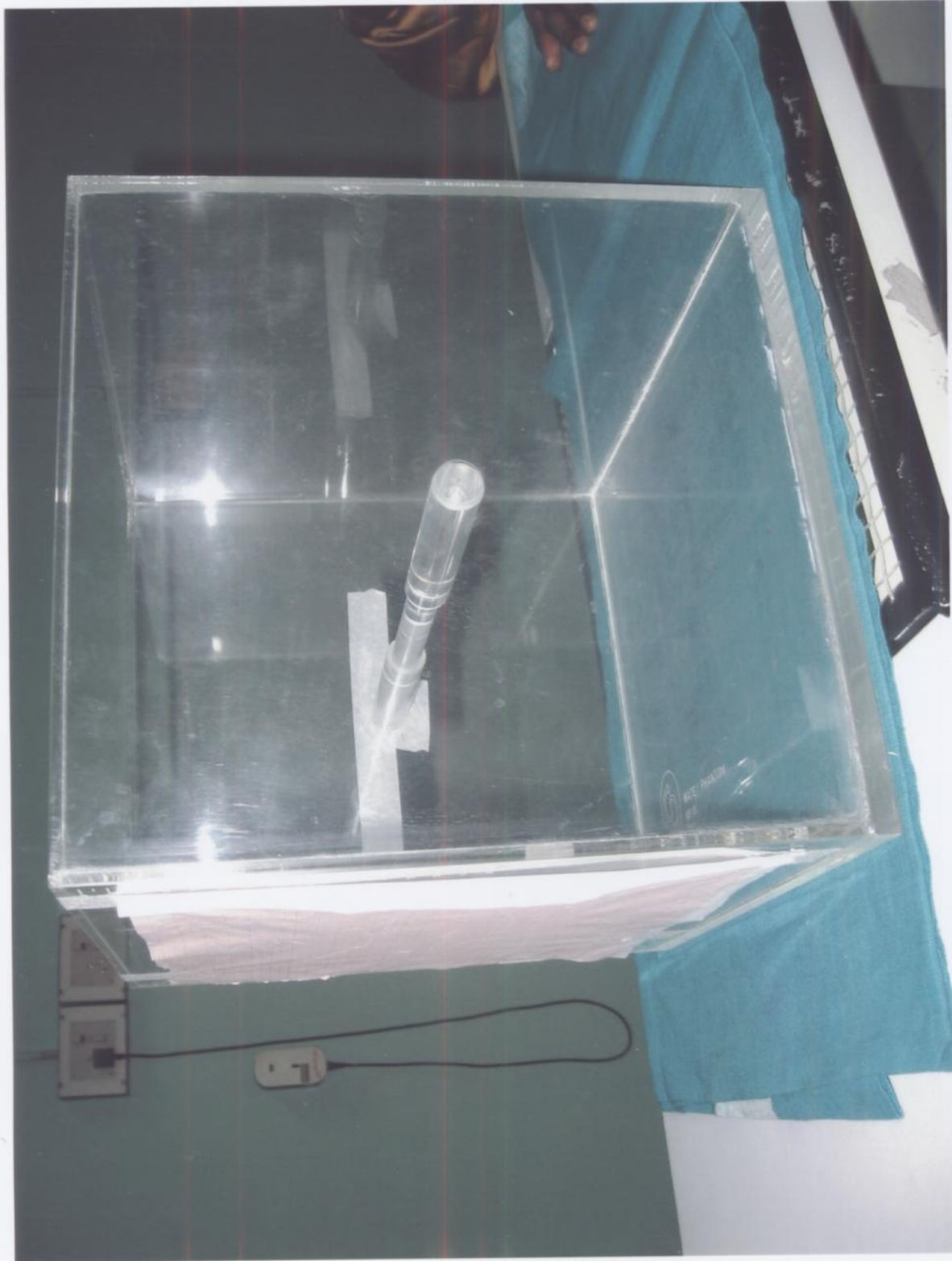
Figure 3 - The water phantom having a volume of 35cmx35cmx35cm is also made by CD high tech
