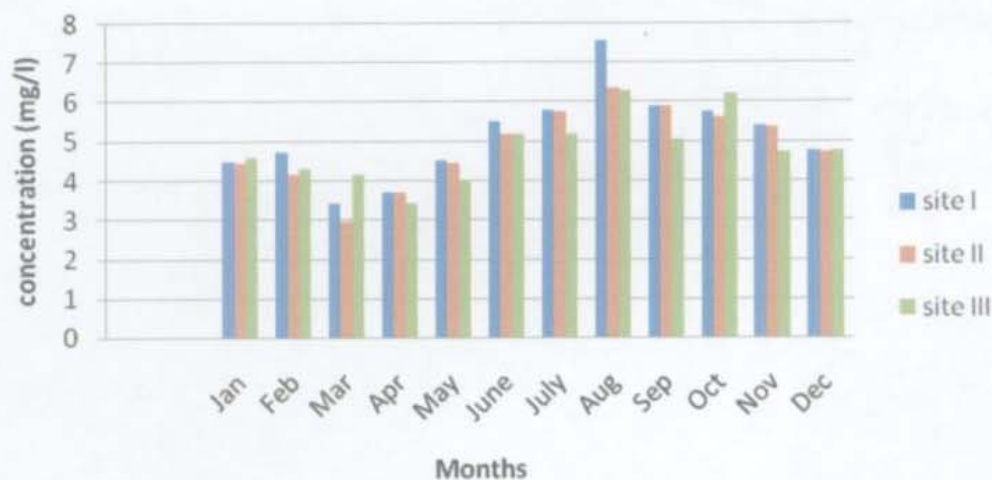
Fig. 15. seasonal variation in the dissolved oxygen content of the three sites during 2004-05
