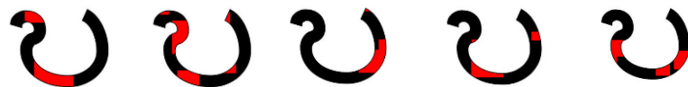
Figure 13 Shows the thickening of the stroke at different regions of the input character pa
