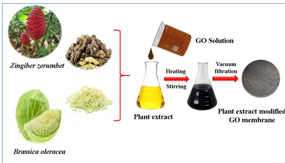
Figure 2.3.2 - Schematic representation of plant extract modified GO membrane synthesis.
