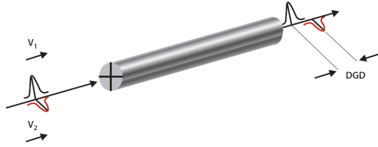
Figure 1.3: Polarization mode dispersion ( http://fobasics.blogspot.com/2012/07/polarization-mode-dispersion.html )
