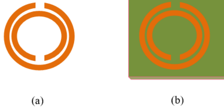
Figure 4.23: Schematic representation of SRRs (a) without substrate (b) on a lossy dielectric (PANI-PTFE/FR3 board/FR4 board) substrate.
