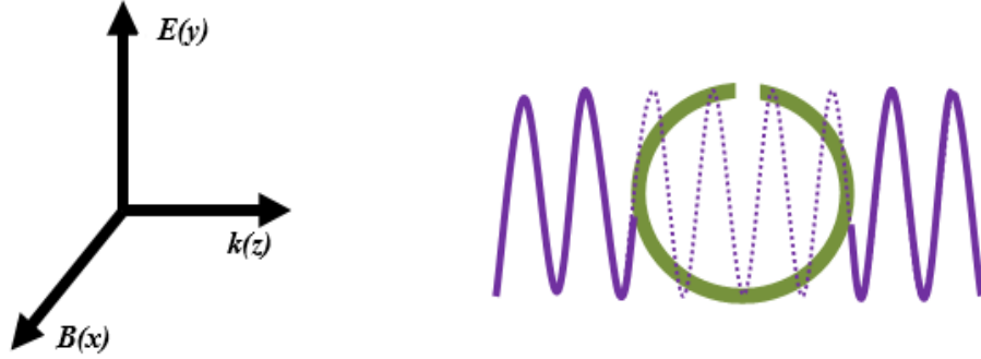
Figure 4.1: Shows the orientation of PANI-PTFE ring in an external EM field.
