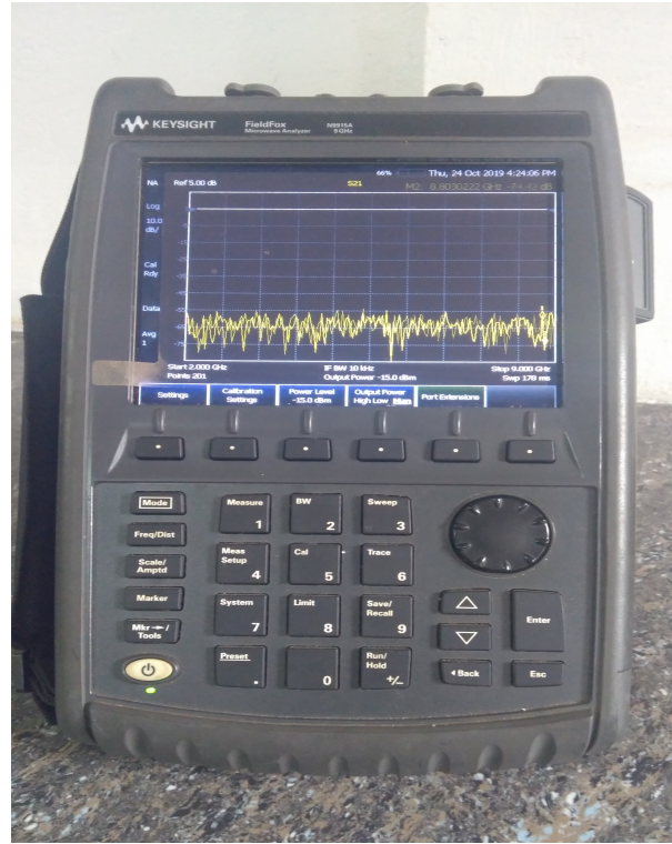
Figure 2.3: Photograph of Vector Network Analyzer used for transmission and reflection measurements.
