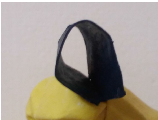
Fig. 1 Photograph of polyaniline–polytetrafluoroethylene (PANI–PTFE) hybrid sheet of thickness 0.9 mm
