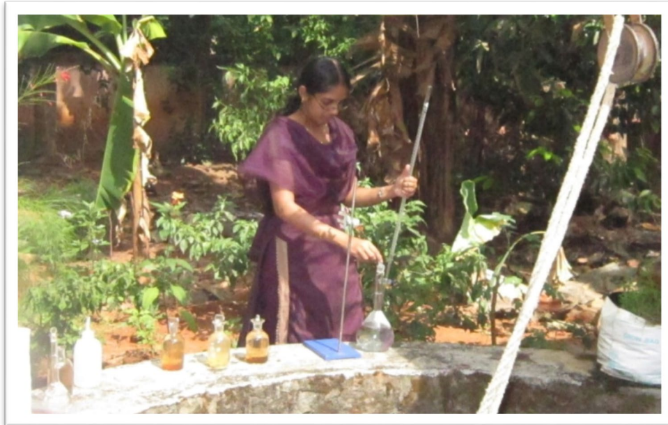
Plate 4.3. Insitu measurement of Dissolved Oxygen content in the well water
