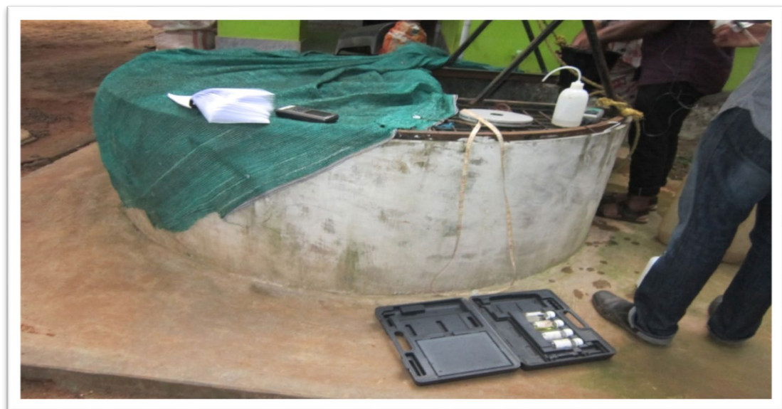
Plate 4.2. Insitu measurement of water quality parameters
