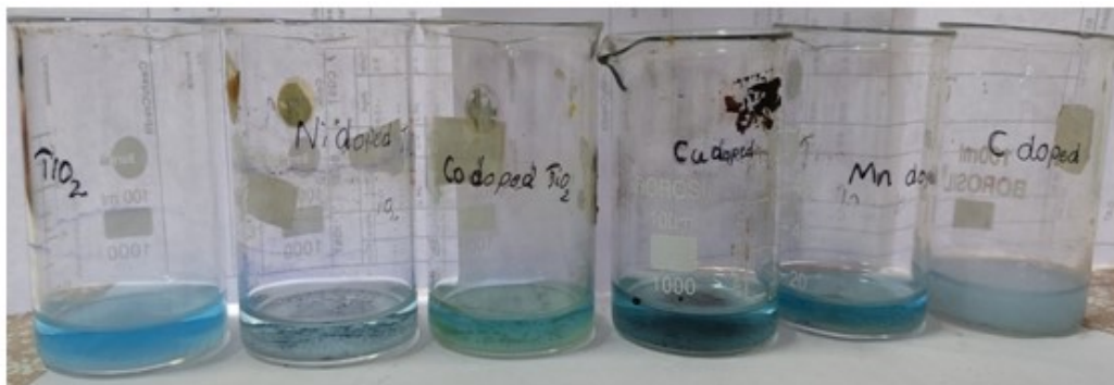
Fig. 3.36 Photograph of dye degradation test of doped and undoped TiO 2 .
