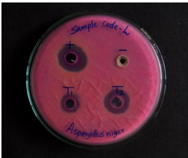
Fig.25. Antifungal assay of 2,4-dihydroxybenzaldehyde N(4)-methyl(phenyl)thiosemicarbazone (denoted as L) on the A. niger
