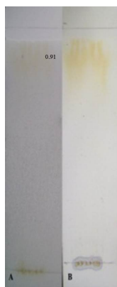
Figure 3.5. TLC of the UNAQE by developing sample (10 \mu\text{g/mL} ) using mobile phase methanol: water: acetic acid (18:9:1 V/ V/ V), and observed under (A) visible light and (B) iodine vapor.
