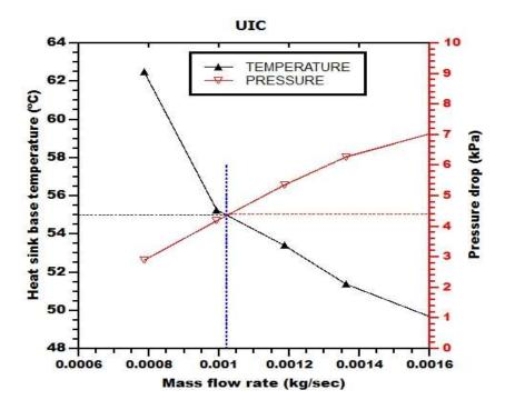
Fig 4.52 Variation of Heat Sink Base Temperature and Pressure Drop with the Mass Flow Rate (UIC)
