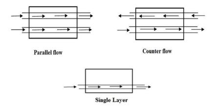
Fig 4.3 Flow Configuration for Experiment Study
