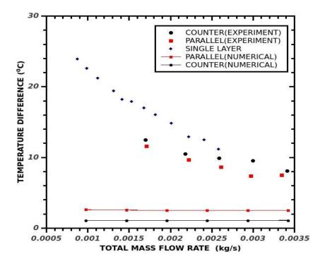
Fig 4.33 Wall Temperature Difference with the Total Mass Flow Rate
