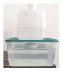
Fig 3.33 Float Chamber with the Reservoir
