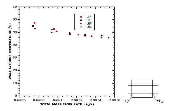
Fig 4.45 Wall Average Temperature with the Total Mass Flow Rate
