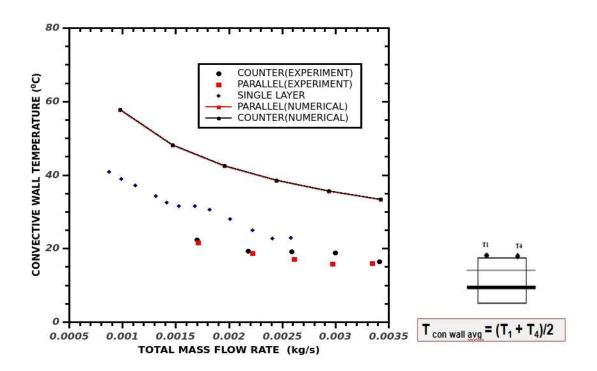
Fig 4.24 Convective Wall Temperature with the Total Mass Flow Rate
