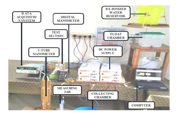
Fig 3.32 Pictorial View of Experiment Setup
