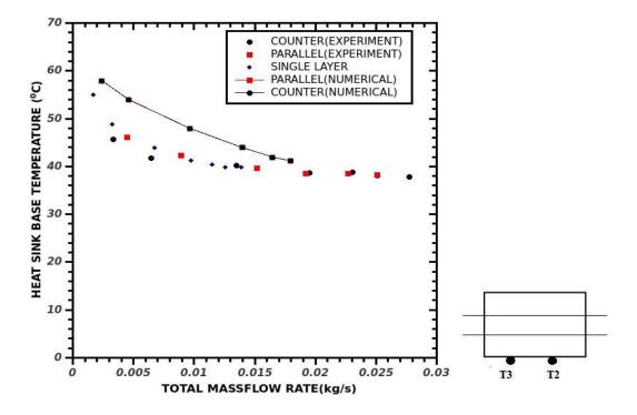
Fig 4.10 Heat Sink Base Temperature Vs the Total Mass Flow Rate
