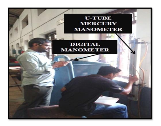
Fig A 2-1, Pictorial view of the digital manometer calibration
