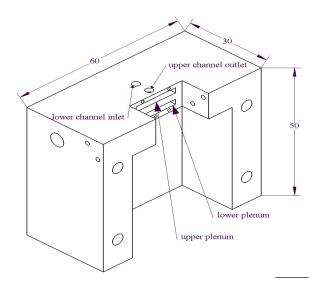
Fig 3.16 Schematic of the Teflon covers
