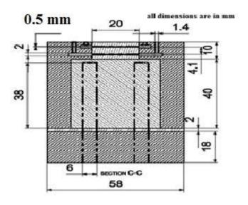
Fig 3.12 Schematic of the Test Piece with Teflon covers
