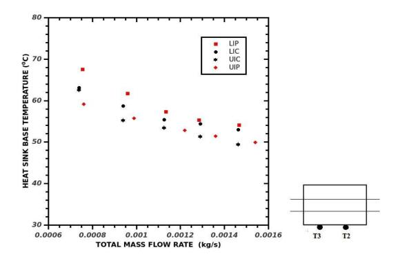
Fig 4.47 Heat Sink Base Temperature with the Total Mass Flow Rate
