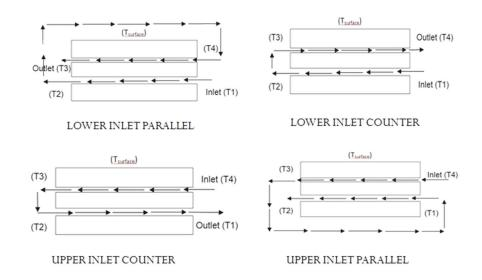
Fig 3.36 Schematic of Different Series Flow Configurations (EXPERIMENT)
