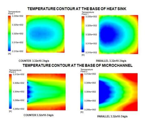
Fig 4.11 Temperature Plot (Case 1)
