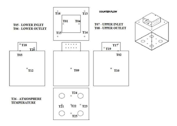
Fig 3.25 Location of Thermocouples in the Test Piece
