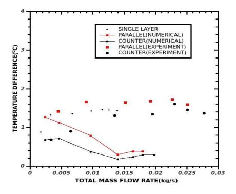
Fig 4.16 Wall Temperature Difference with the Total Mass Flow Rate
