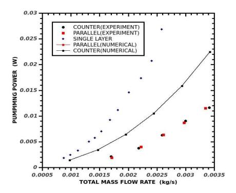
Fig 4.22 Pumping Power with the Total Mass Flow Rate
