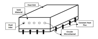
Fig 1.3 Example for Single Layer Microchannel
