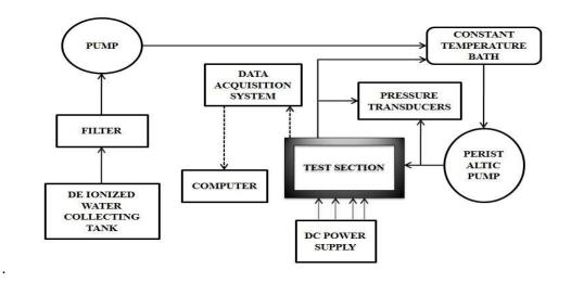
Fig 3.5 Schematic Diagram of the Experiment
