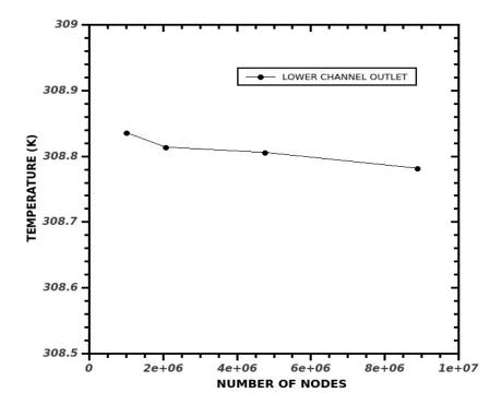
Fig 4.2 Lower Channel Outlet Temperature Vs Number of Nodes
