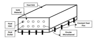
Fig 1.4 Example for Double Layer Microchannel (CF)
