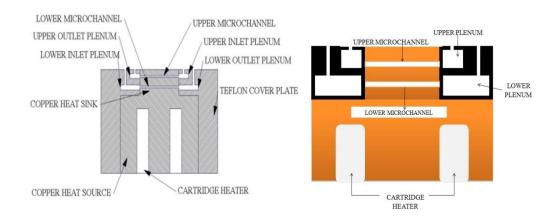
Fig 3.13 Sectional view of the Test Piece with Teflon covers.
