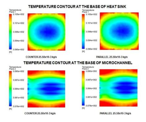
Fig 4.15 Temperature Plot (Case 5)
