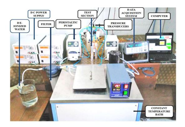
Fig 3.6 Photograph of Typical Experiment Setup
