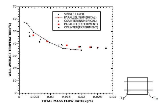
Fig 4.9 Wall Average Temperature Vs the Total Mass Flow Rate
