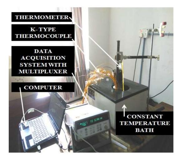
Fig A1 – 1, Pictorial view of the Thermocouple Calibration
