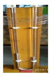
Fig 3.34 U- Tube Manometer
