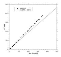
Fig A 2-3, Digital manometer calibration curves
