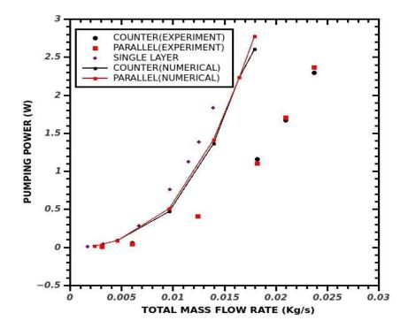
Fig 4.6 Pumping Power Vs the Total Mass Flow Rate
