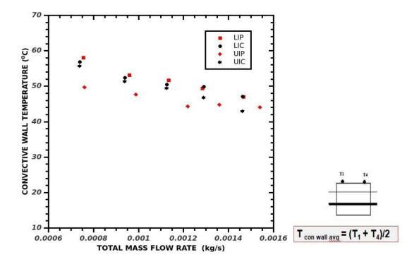
Fig 4.46 Convective Wall Temperature with the Total Mass Flow Rate
