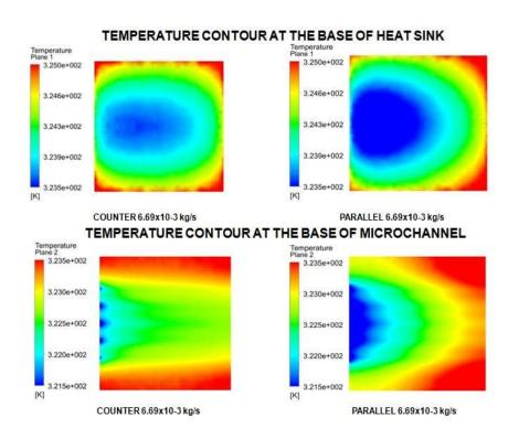
Fig 4.12 Temperature Plot (Case 2)
