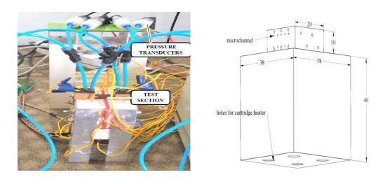
Fig 3.7 (a) Test section and Pressure Transducers
