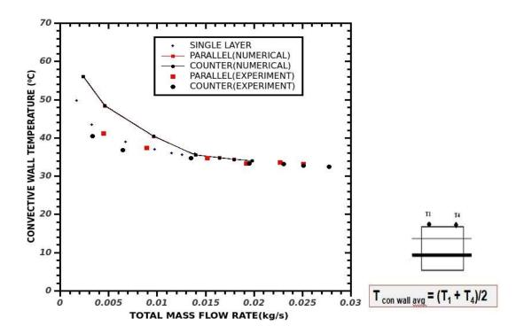
Fig 4.8 Convective Wall Surface Temperature with the Total Mass Flow Rate
