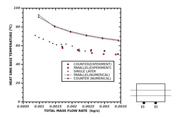
Fig 4.26 Heat Sink Base Temperature with the Total Mass Flow Rate
