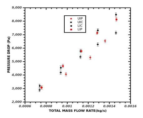
Fig 4.40 Pressure Drop with the Total Mass Flow Rate
