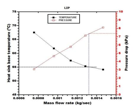
Fig 4.49 Variation of Heat Sink Base Temperature and Pressure Drop with the Mass Flow Rate (LIP)
