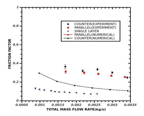
Fig 4.21 Friction Factor with the Total Mass Flow Rate
