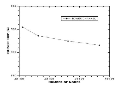
Fig 4.1 Lower Channel Pressure Drop Vs Number of Nodes
