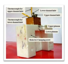
Fig 3.15 Photograph of the Teflon Cover used in the Experiment.
