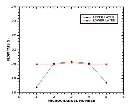
Fig 4.36 Flow Rate Vs Microchannel Number (PF)
