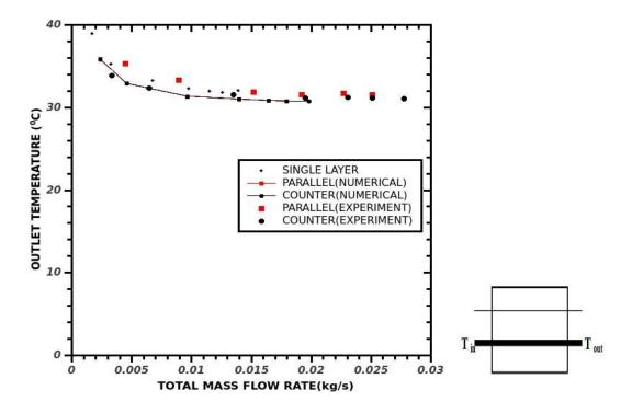
Fig 4.7 Outlet Temperature Vs the Total Mass Flow Rate
