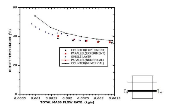
Fig 4.23 Outlet Temperature with the Total Mass Flow Rate
