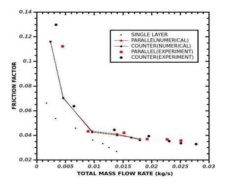
Fig 4.5 Friction Factor Vs the Total Mass Flow Rate
