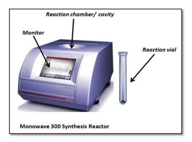
Figure 2.1: Microwave reactor (Anton Paar monowave-300)
