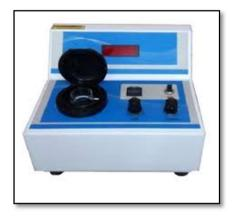
Figure 5.9: Image of Turbidimeter used for quantification of Pb2+ ions(LABTRONICS LT-33 Digital Turbidity Meter)
