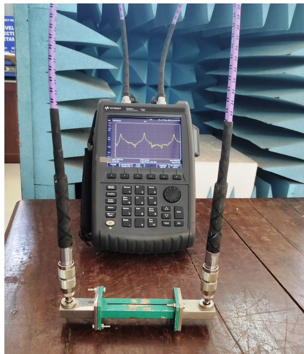
Figure 4.9: Cavity resonator connected to transmitting and receiving probes of Vector Network Analyser.
