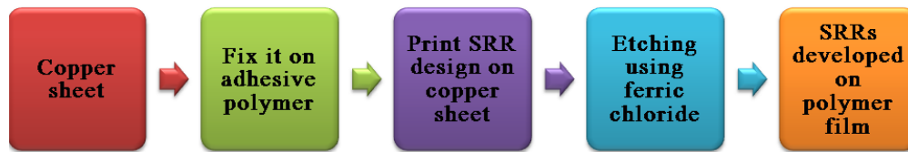
Figure 2.11: Flow diagram representing the various steps of direct printing method.
