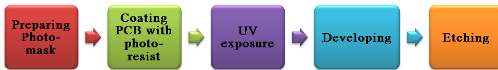
Figure 2.4: Block diagram representing the various steps of photo chemical etching method.
