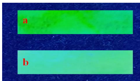
Fig.20 Photographic image under UV-light (a) PMB3 aggregates formed in DMF-Water mixture of water fraction 90% (fw =90%) coated on filter paper (b) PMB3 aggregates coated filter paper dropped with \text{Cu}^{2+} ion
