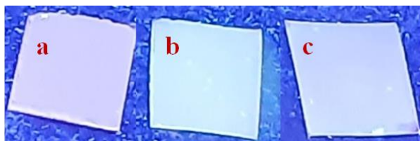
Fig. 15. Photographs of TLC plate containing (a) TLC plate only (b) TLC plate coated with PMB3 aggregates (c) TLC plate coated with PMB3 aggregates and PA.
