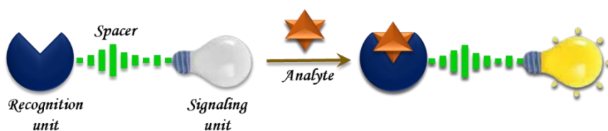
Fig.3 Schematic representation showing binding of analyte by a fluorescent chemosensor
