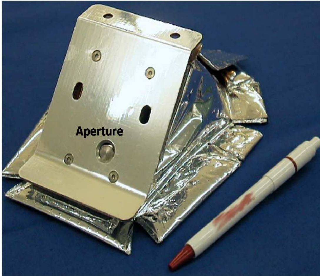
FIGURE 2.13: X-ray Solar Monitor. The aperture through which x-rays reach the detector, is marked (the closed shutter can also be seen)
