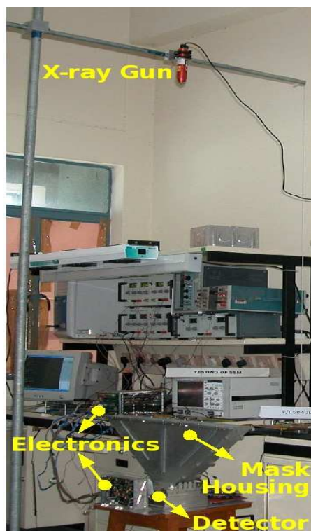
FIGURE 3.29: Experimental set-up showing the detector with the coded-mask and the source held at a certain height with a pole
