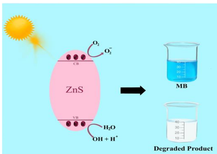
Figure 3.9- Schematic illustration of the dye degradation process using ZnS
