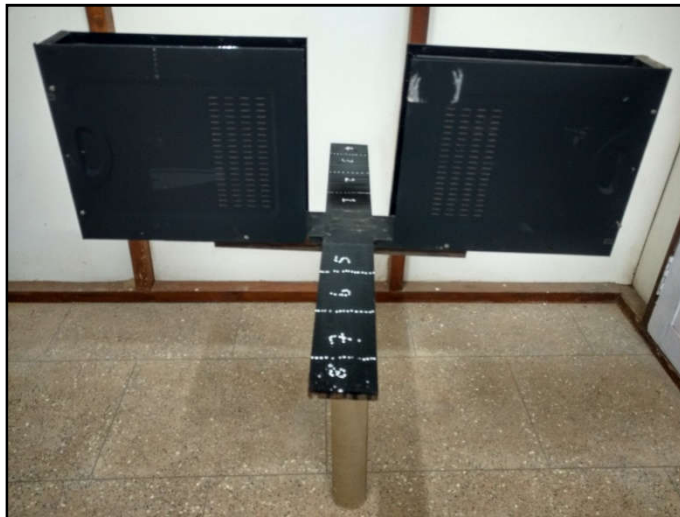
Figure 3.5: Elevated plus maze apparatus.
