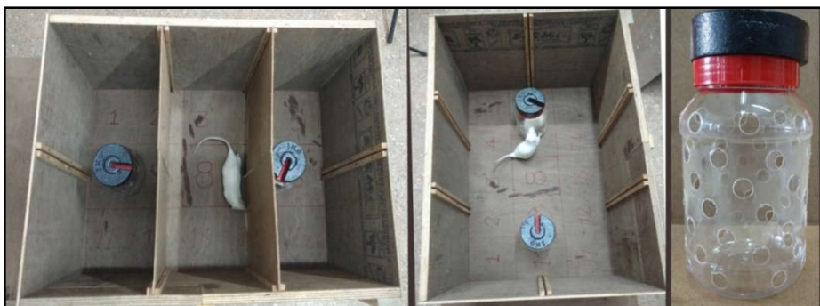
Figure 3.9: Three chamber Sociability and social novelty test apparatus.
