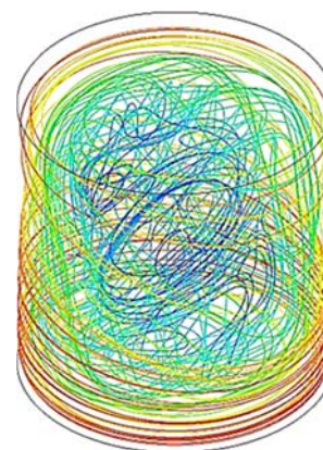
Fig. 6.21. Streamlines of fluid flow for glycerine/water system
