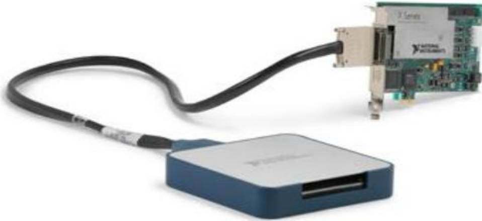
Figure.7.2 PCIe-6351 Multi-function I/O device and Data Acquisition (DAQ) card and connector cable and connector block
