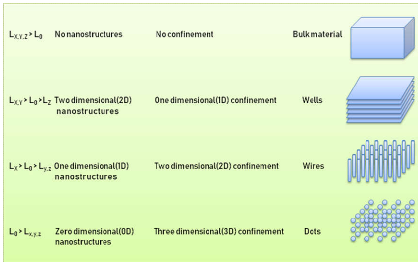
Figure 1.6. Schematic description of the confinement effects in different dimensions (adapted from Fundamentals of nanomaterials, Lecture 5, Nanomaterials).
