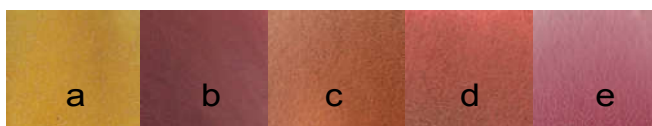
Figure 3.5. Photographic images of the cellulose papers deposited with various metal and alloy nanoparticles: (a) Ag; (b) AgAu (7:3); (c) AgAu (5:5); (d) AgAu (3:7); and (e) Au. The corresponding diffuse reflectance UV-Vis absorption spectra are presented above.
