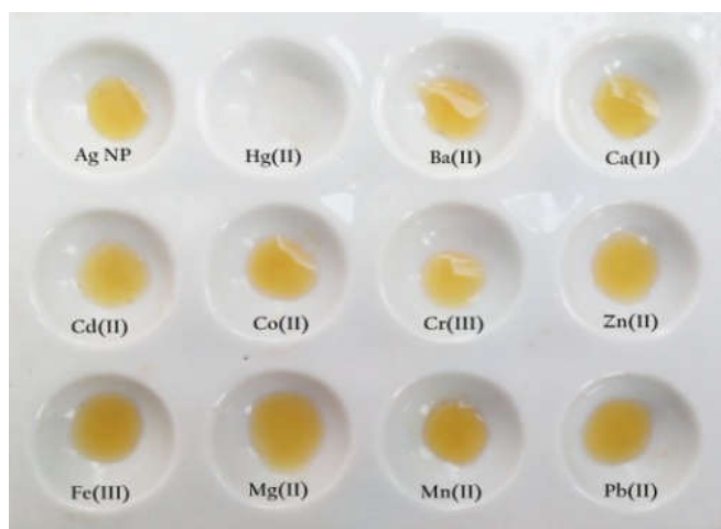
Figure 4.4: Optical response of the aqueous dispersion of Ag NPs with the various metal ions.
