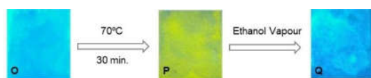
Figure 4. Solid state Fluorescence of Ugi EML BLUE: O) an air dried film made by drop casting an ethanol solution of Ugi EML BLUE on a glass substrate. P) Yellowish-green fluorescence showed by film O when subjected to thermal annealing at 70°C for 15 minutes. Q) Reinstating the bluish fluorescence by ethanol vapour etching.
