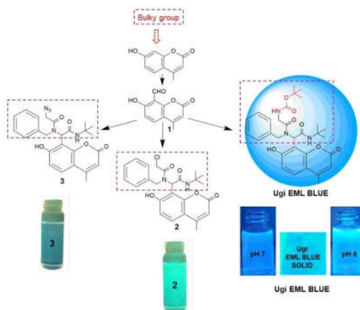
Figure 1. Structure of coumarin derivatives and their Photoluminescence under UV light
