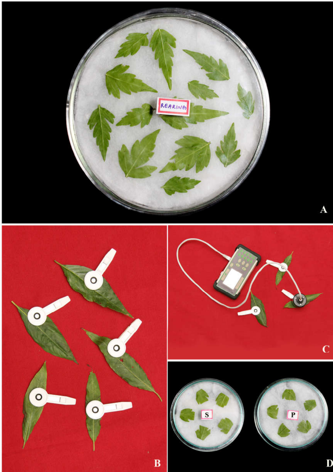
A. Rearing of mites under laboratory condition; B. Chlorophyll Fluorometer (Handy PEA); C. Leaf samples kept in leaf clips for dark adaptation; D. Leaf disc method for breeding biology study
