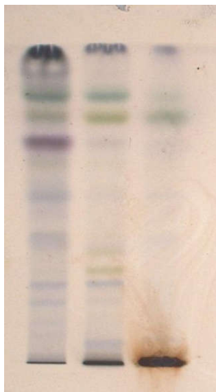
Figure-3.11: HPTLC image after derivatization observed at 550nm.
